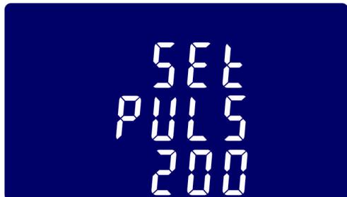
From the Set-up menu, use **M ↑** and **P ↓** buttons to select the Pulse width option.
