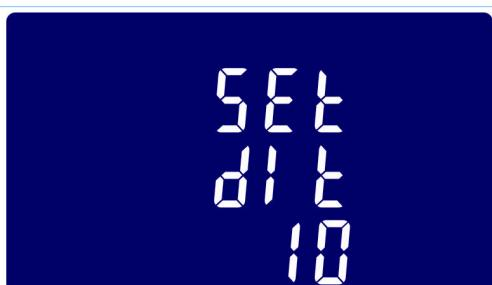
From the set-up menu, use and buttons to select the DIT option. The screen will show the currently selected integration time.
